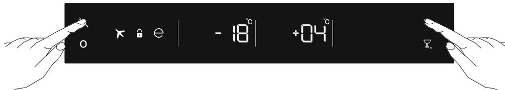
Press on Freezer and Cooler buttons simultaneously for 5 seconds.
