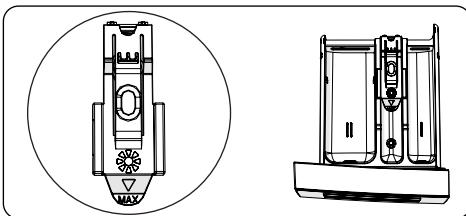
This compartment is for softeners, conditioners or starch. Follow the instructions on the packaging. If softeners leave residue after use, try diluting them or using a liquid softener.
