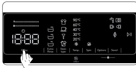
You can use this auxiliary function to delay the start time of the washing cycle for 1 to 23 hours. To use the delay function:
