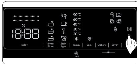
By pressing on the Start/Pause button, you may start the programme you have selected or suspend a running programme. If you switch your machine to the standby mode, the Start/Pause led on the electronic display will blink.
