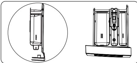
This compartment should be used only when the pre-wash feature is selected. We recommend that the pre-wash feature is used only for very dirty laundry.
