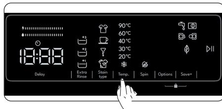
You can use the washing water temperature setting key to set the temperature of the washing water for your laundry.
