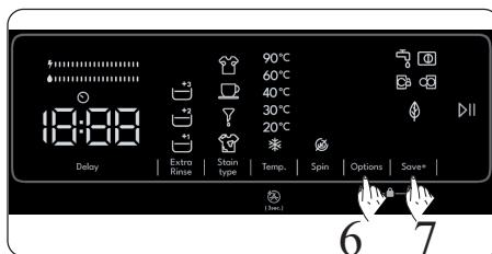
If any button is pressed or selected programme is changed by the programme dial while the child lock is active, the “CL” symbol will flash on the electronic display for 2 seconds.
