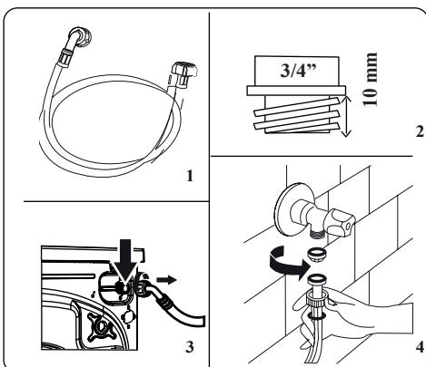
1. Your machine may have either a single water inlet connection (cold) or double water inlet connection (hot and cold) depending on the machine specifications. The white capped hose should be connected to cold water inlet and red capped hose to the hot water inlet (if applicable).
