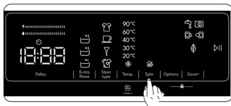
You can press the spin speed setting key to decrease the spin speed gradually between the selected program's maximum spin speed and the spin cancelled ( ⚡ ) option.
