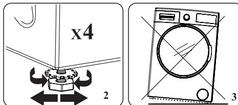
2. To increase the height of the machine, turn the feet clockwise. To decrease the height of the machine, turn the feet anticlockwise.
