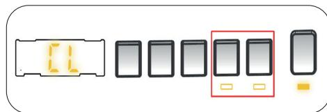
If any button is pressed or selected programme is changed by the programme dial while the child lock is active, the “CL” symbol will flash on the electronic display for 2 seconds.
