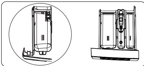
This compartment is for liquid or powder detergents or limescale remover. The fluid detergent level plate will be supplied inside your machine. (\*)
