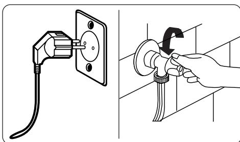
Turn your mains power supply off and remove the plug from the socket before carrying out maintenance and cleaning of your machine. Turn off the water supply before starting maintenance and cleaning of your machine.
