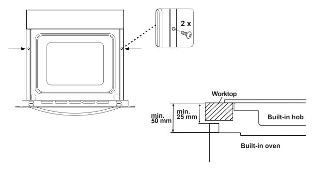
If the oven is installed under a hob, the distance between the worktop and the top panel of the oven must be minimum 50 mm and the distance between the worktop and the top of control panel must be minimum 25 mm.
