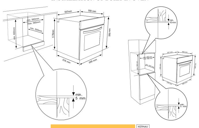
Insert the oven into the cabinet by pushing it forward. Open the oven door and insert 2 screws in the holes located on the oven frame. While the product frame touches the wooden surface of cabinet, tighten the screws.
